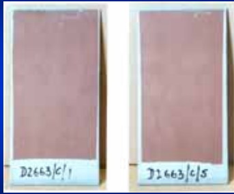
Interplate 855 @ 15µm (0.6 mil) dft
